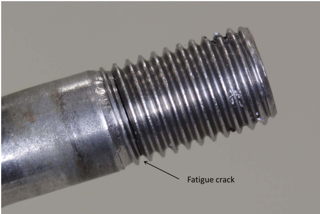
Figure A3: Forward fuselage lateral tie rod showing right side thread with fatigue crack
