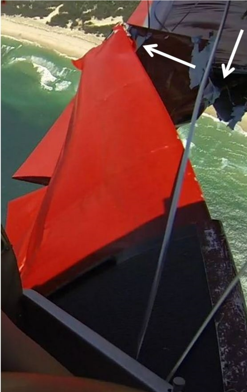
Figure 19: +0.336 sec - front spar fractures
