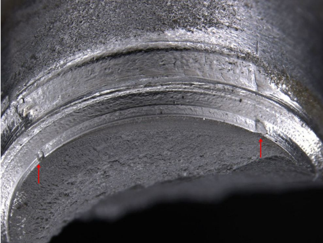
Figure A5: Thread irregularities at fatigue crack origin
